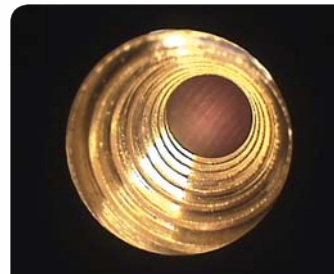
Well cutted inner threads in hollow shaft for precision clocks
