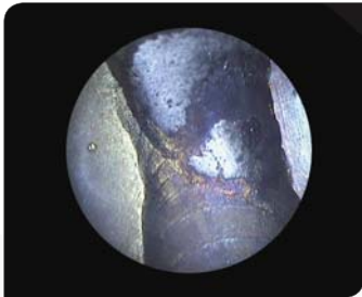
Run-out of a welded seam
