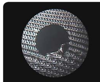
Metal filter with material covering at the end part of the filter before beading
